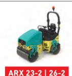
Operating weight: 2085–2350 kg (4600–5040 lb) Maximum weight: 2285–2550 kg (5180–5620 lb) Drum width: 1000–1200 mm (39.4–47.2 in) Max working offset mode: 40 mm (1.57 in) Engine: Kubota – 25 kW (33.5 HP) EU Stage V/U.S. EPA Tier 4f Kubota – 24.8 kW (33.3 HP) EU Stage IIIA/U.S. EPA Tier 4i
