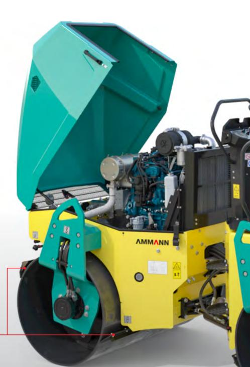
DRUM SCRAPERS Two scrapers per drum is standard.
