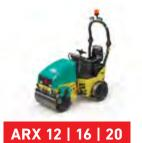
Operating weight: 1460–1550 kg (3220–3420 lb) Maximum weight: 1610–1700 kg (3550–3750 lb) Drum width: 820–1000 mm (32.3–39.4 in) Max working offset mode: 50 mm (1.97 in) Engine: Yanmar – 14.6 kW (19.6 HP) EU Stage V/U.S. EPA Tier 4f Yanmar – 15 kW (20.4 HP) EU Stage V/U.S. EPA Tier 4i
