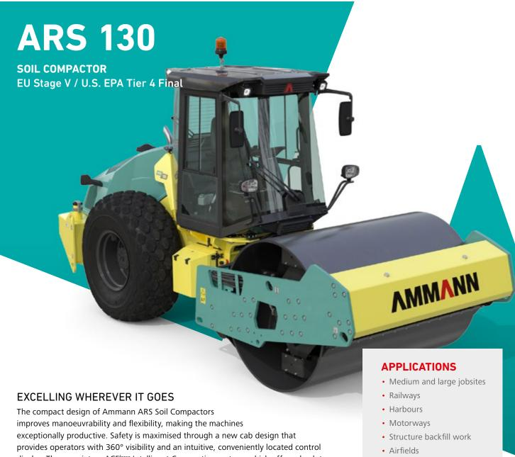
display. The proprietary ACE<sup>force</sup> Intelligent Compaction system, which offers absolute compaction measurement and optional documentation, improves efficiency and quality. The availability of a wider range of centrifugal forces make the machine a perfect fit for many applications and varied materials.
