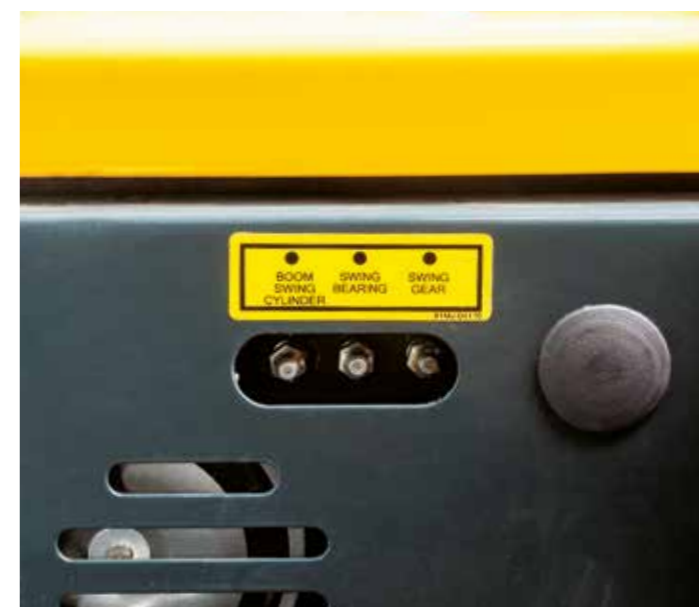
Centralised grease points Grease fittings are centralised in one lubrication bank for quick, easy servicing.
